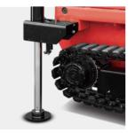
Equipped with one key outrigger leveling function, automatically adjust the frame to the level state, hydraulic outrigger to enhance the stability of the equipment. At the same time, it can also operate a single outrigger to meet the operation requirements under special working conditions.
