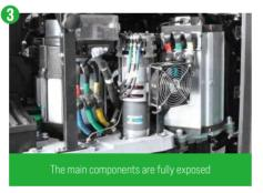
The seat can be turned open at a large angle, which is convenient for maintenance work.
